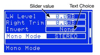
The LWLevel and Right Trim above are typical sliders. When one of them is selected, tap the wheel to adjust its value. Then turn the wheel to raise or lower the value, on the screen that appears. When you're satisfied with the change, tap again to return to the previous menu.
