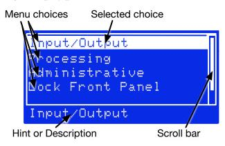
In this example, you'd turn the wheel to highlight one of the lines. If there are more choices than can be displayed at once on the screen, a scroll bar helps you keep track of vertical progress through the choices.
