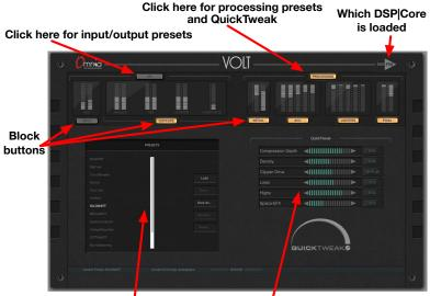
Preset list or high res meters Function or QuickTweak controls
